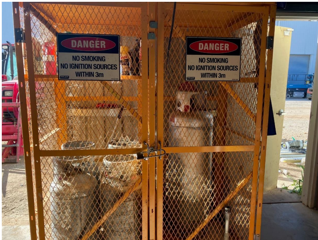
Figure 10: Combustible Chemicals kept banded and caged
